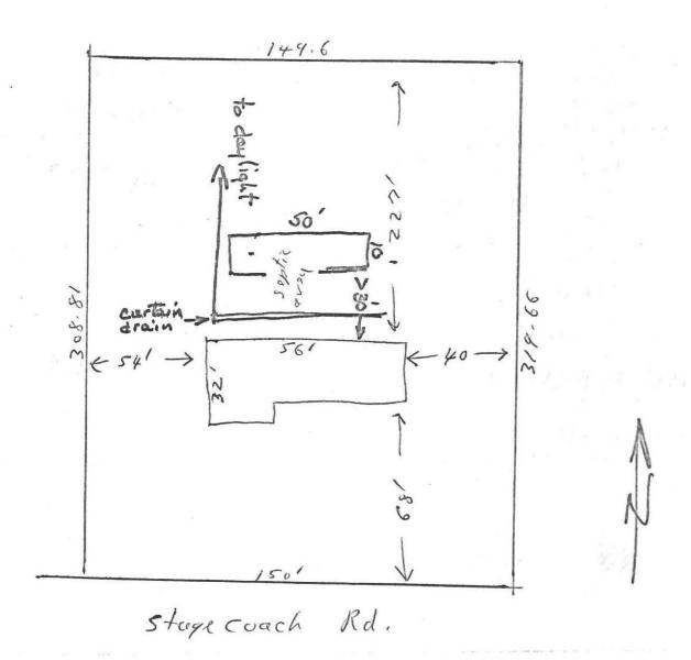
Curtain drain to be installed at least 6.0" below natural ground or 4.0' below top of ground cet base of disposal bed.
