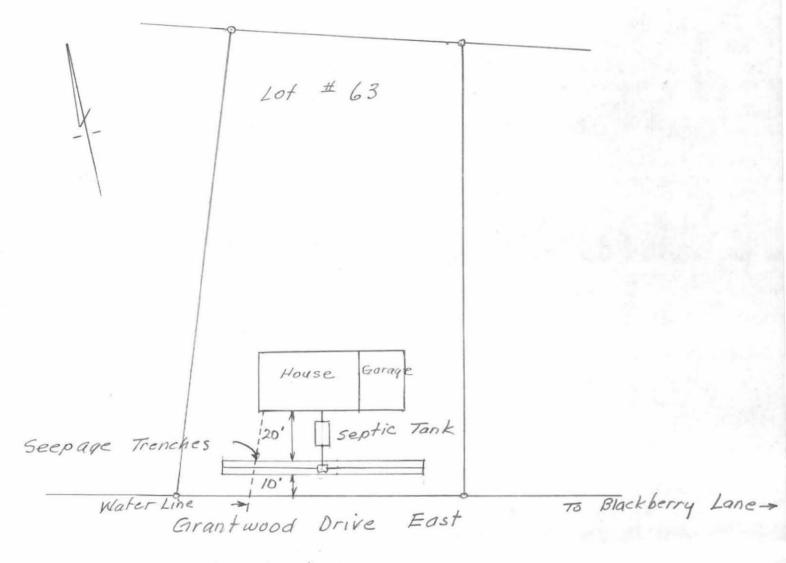
Note: Encase waterline in 6" of concrete for 5" on each side of disposal seepage trenches.
