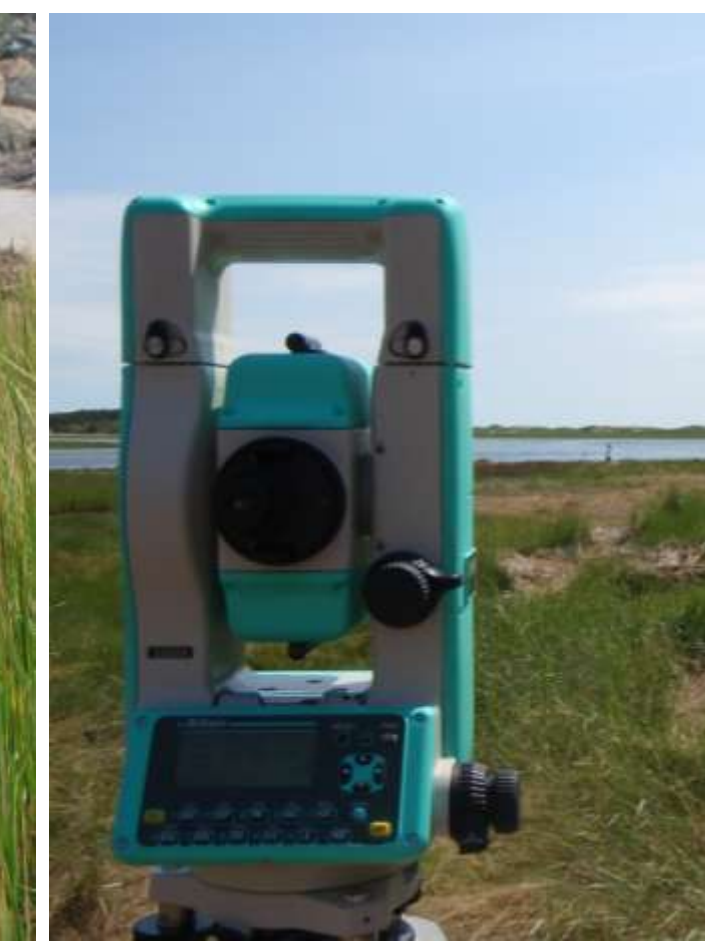
Nikon DTM 550 Total Station used for surveying the marsh
