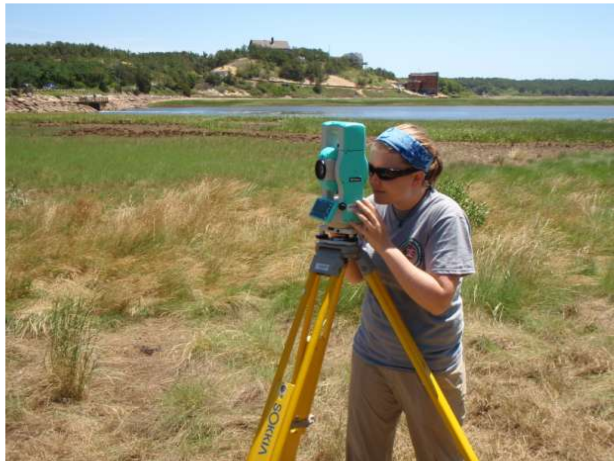
Using the total station to record the survey points and the vegetation type at each point.
