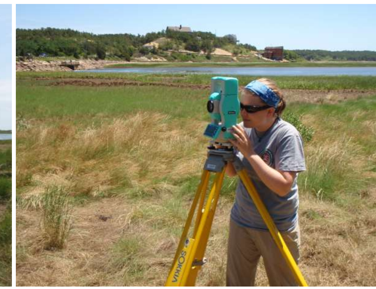
Using the total station to record the survey points and the vegetation type at each point.
