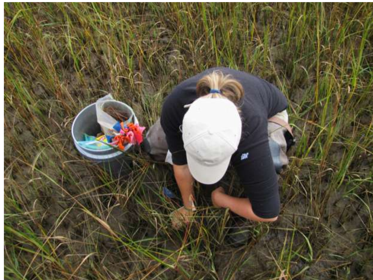
Photo Credit: Anne Ribereau-Gayon Placing flags as guides for survey lines.
