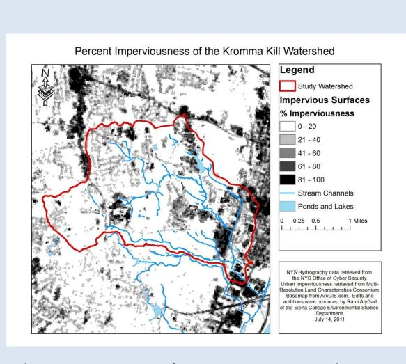
The impervious surfaces map is a good starting point for extracting possible sources of increased runoff flows. When observing this map, we see that there are a handful of areas that are fifty plus percent impervious. These highly impervious areas include the following: Siena College, East Hills Residential Development, Lakeshore Apartment Residential Development, Altech Steel Plant, and much of Menands (which is built on the Hudson River flood plain).
