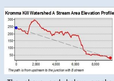
The above and below graphs represent the Stream Area Elevation Profile for the North and South stream branches located within the Kromma Kill Watershed. The Northern stream (Stream A) has a higher peaks and slopes at larger distances from the outlet compared to the Southern stream (Stream B), which has a more gradual decline in elevation as it approaches the outlet.
