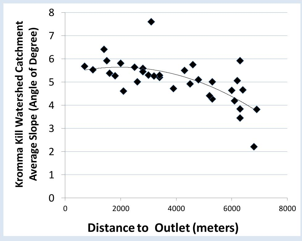
The above graph displays the analysis of average slope for the various subbasins located at different distances from the watershed outlet. Average slope has lower values at greater distances from the watershed outlet.
