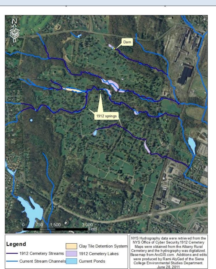
channel. In 1912, there were multiple holding ponds/lakes that slowed down flows. Furthermore, the 1912 channels were meandering in nature and have been out through development over the past century.
