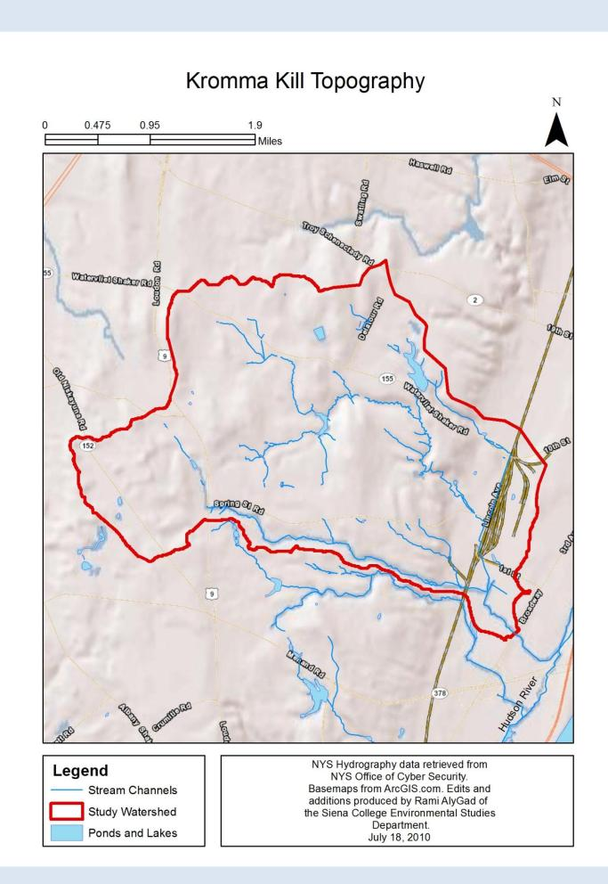
The topographic map (left) shows us that there is a steep slope in the downstream portion of the watershed. This slope can exacerbate flooding and stream bank
